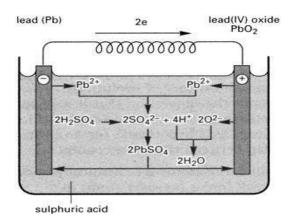
The cell represented as  $Pb,\,PbSO_{4}$   $_{(s)}$  /  $H_{2}SO_{4}$  (30%) /  $PbO_{2}$   $_{(s)}$  , Pb
